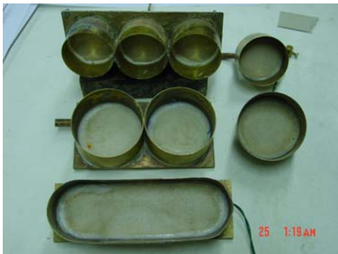
Fig. 14 Photograph of different caisson types used to examine the effect of the shape.
